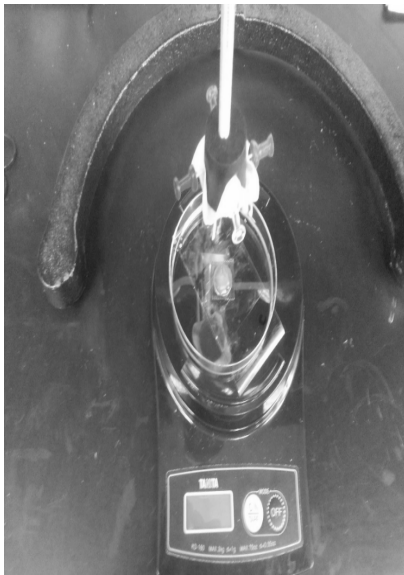
Figure 1: The wiping apparatus to test the effect of Octenidine Hydrochloride (OH) wiping on Clostridioides difficile spores inoculated on stainless steel discs. Rotations per minute were controlled by the rotating bar settings and pounds of pressure were controlled by the weigh balance.
