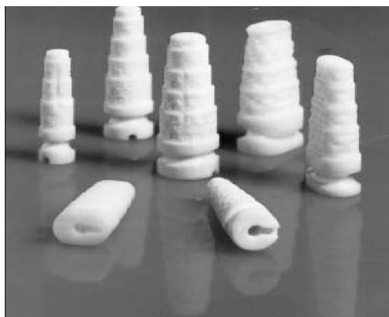
Figure 4: Dental implants made of alumina [35].
