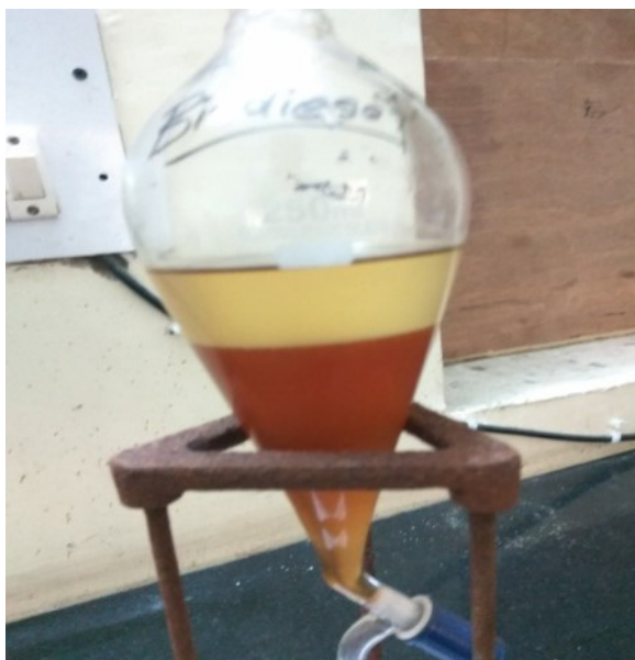
Figure 4: Separation of biodiesel from glycerol.
