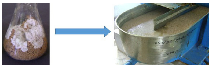
Figure 2: The deinking of paper pulp during pulping process in a beater machine. Fungal enzymes produced in solid state fermentation extracted and added to beater just after the initial pulping.
