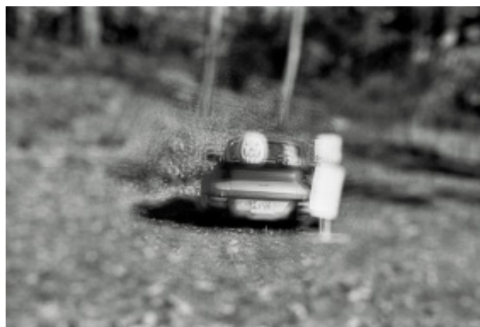
Figure 6: Photograph with the modified lens at F/8. At this F-stop the diameter of the lens aperture is 6.25mm and a fairly large amount of over refracted light still reaches the film plane. Note that the central image has improved enough to make the letters of the license plate almost distinguishable.
